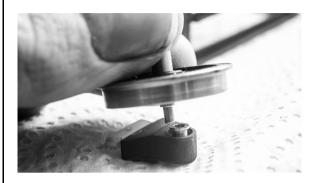
The bearings should be pressed into place using the axle as a drift to help. It should also be noted that 3 Ton Slate wagons require the bearing seat to be drilled further in order that the bearing is recessed as far
