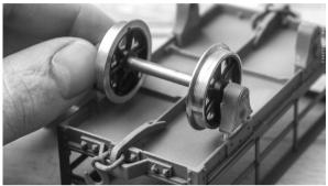
the wagon body (don't forget the wheels!) and then passing a 1mm drill bit through the 3 holes in the solebar and through the axlebox. Into this hole can now be glued the 3 square headed fixing pins. You could use a length of 14BA stud and a nut
